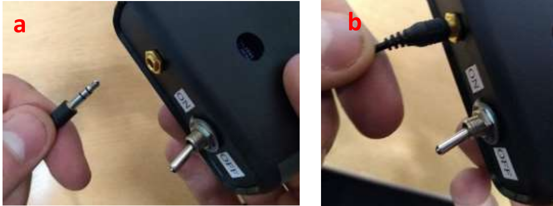
Figure 4: Audio jack, a) Before connecting, b) After connecting
